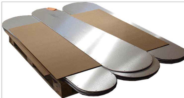
*The strength of the automotive market and other industries investing in robotics has Weaver busy fabricating parts for Fanuc America. Shown are laser-cut aluminum blanks that Weaver forms and powder-coats.*
