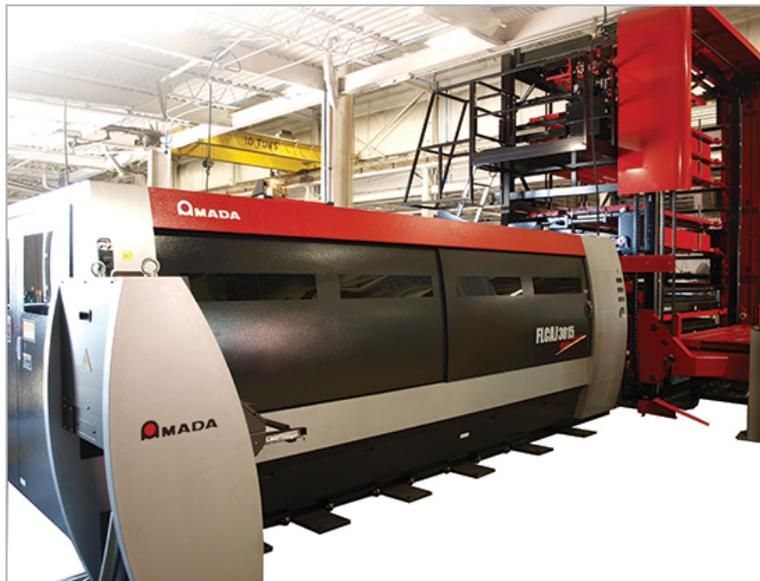
*Weaver Fab & Finishing's new 2-kW fiber-laser cutting machine cuts aluminum and other reflective materials extremely efficiently, and it will cut mild steel four to five times faster than the firm's aging 2-kW CO<sub>2</sub> machine. Key to its success is the automated material-storage tower that "changes how we buy our materials," says Jim Lauer. "We can schedule more accurately and predictably and minimize or even eliminate deviations from our planned production schedules."*
