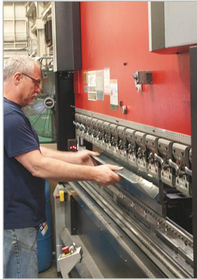
*Accompanying the new fiber-laser cutting machine at Weaver is this Amada servo-hydraulic press brake. Its thickness-detection system automatically adjusts the entry depth of the forming tool based on sheet thickness.*
